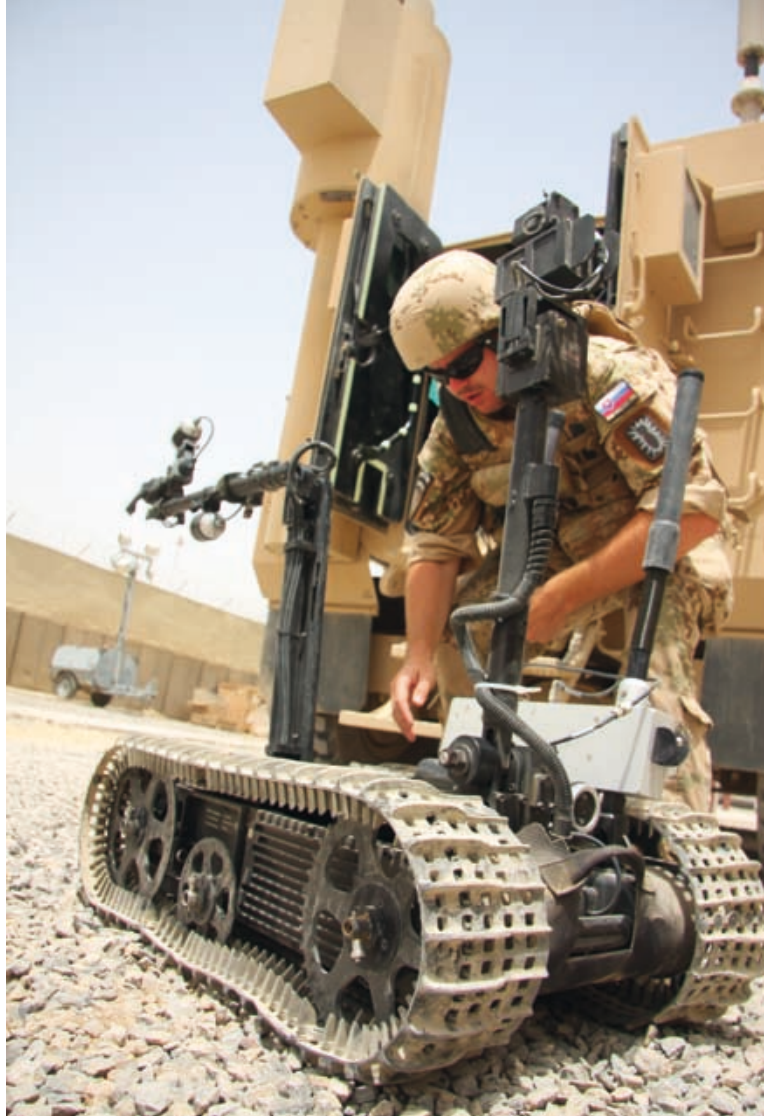
An EOD specialist with a robot for reconnaissance and disposal of improvised explosive devices
